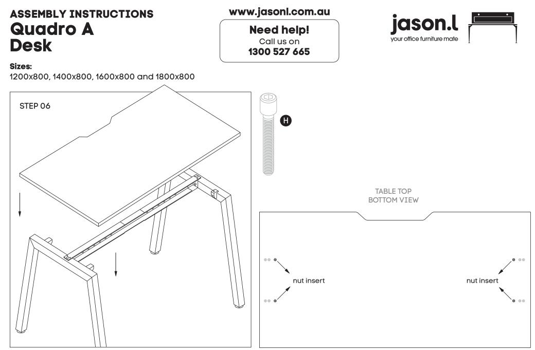
Place desktop ontop of frame - with cutout at the back of the desk. Nut inserts in top will align with plastic joiner brackets using M6x30MM (H) sockets attached top to frame.
