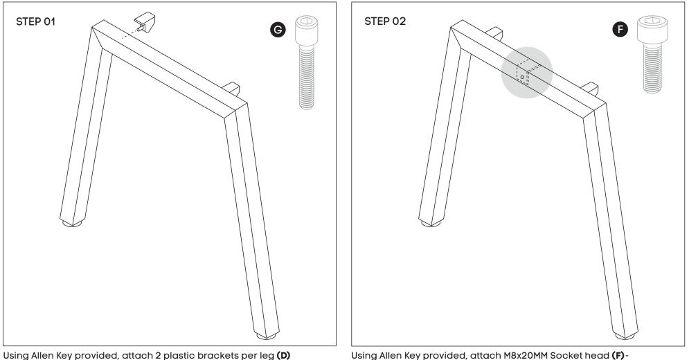
screw socket half way into leg for both legs (B)
