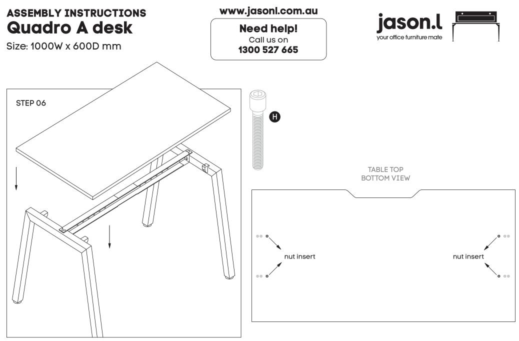
Place desktop ontop of frame. Nut inserts in top will align with plastic joiner brackets using M6x30MM **(H)** sockets attached top to frame.
