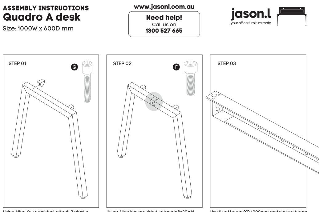
Using Allen Key provided, attach 2 plastic brackets per leg **(D)** (as per picture above) using M6x20MM **(G)** Socket head screw Using Allen Key provided, attach M8x20MM Socket head **(F)**- screw socket half way into leg for both legs **(B)**  Use fixed beam **(C)** 1000mm and secure beam using screws provided to suit 1000mm desk
