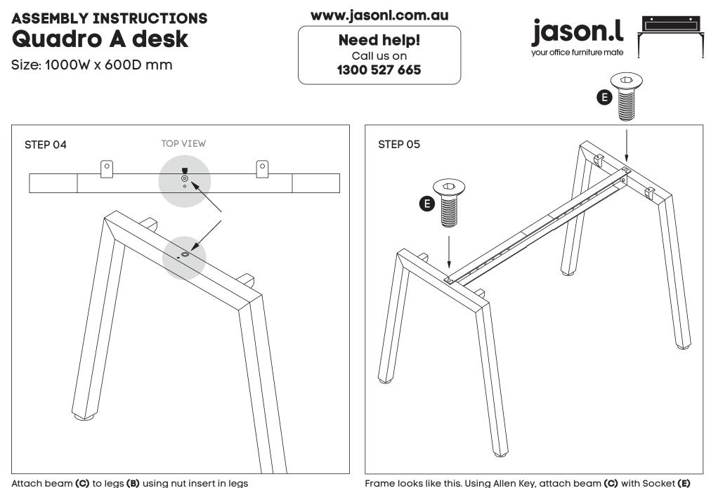
Attach beam **(C)** to legs **(B)** using nut insert in legs See point attached
